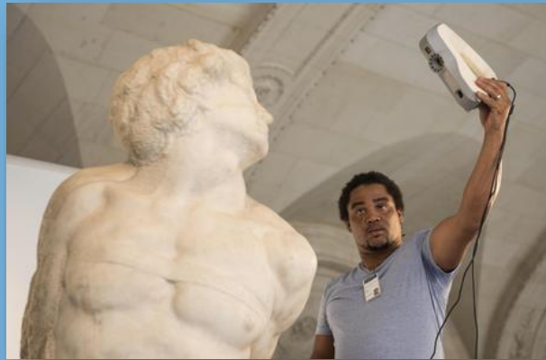
Laser scanning of Michelangelo's prisoners in the Louvre in Paris
